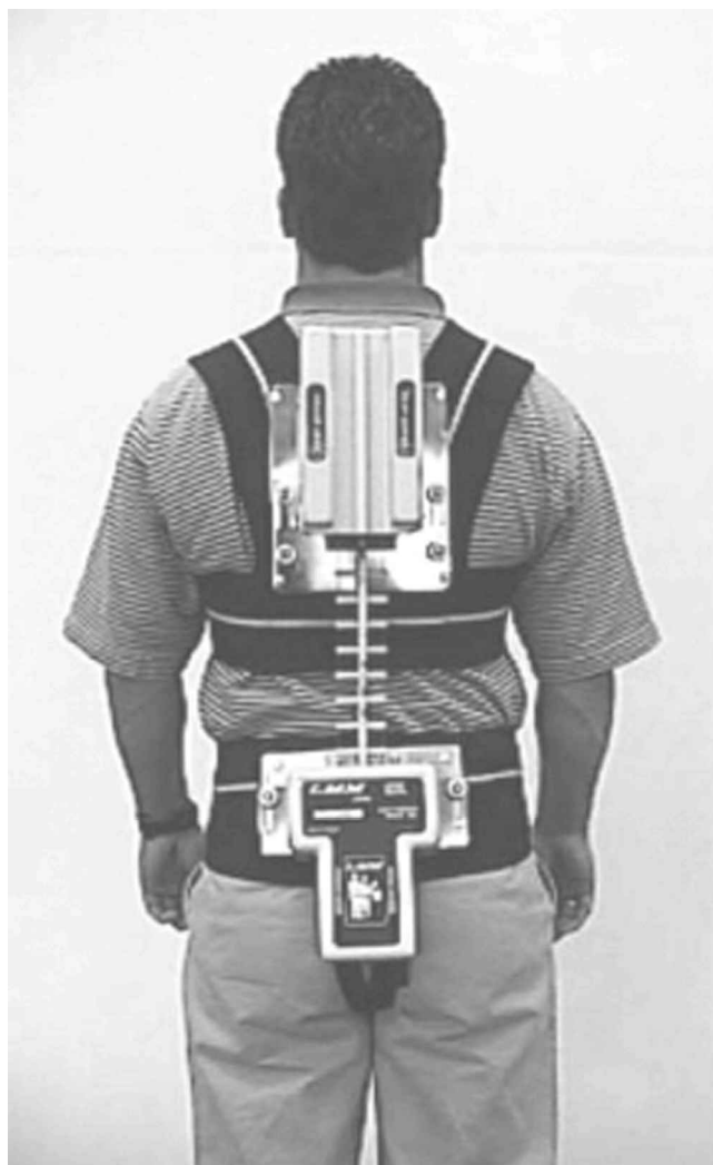
Fig. 1. The Lumbar Motion Monitor (Wellness Design™, Chattanooga Group, Inc., Hixson, TN).
